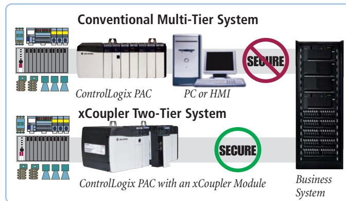
Comparison of a typical plant floor multi-tier system versus the xCoupler two-tier system
