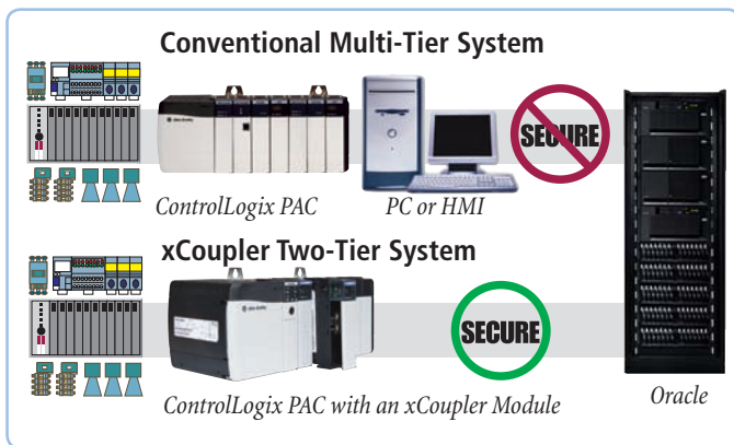
Comparison of a typical plant floor multi-tier system versus the xCoupler two-tier system
