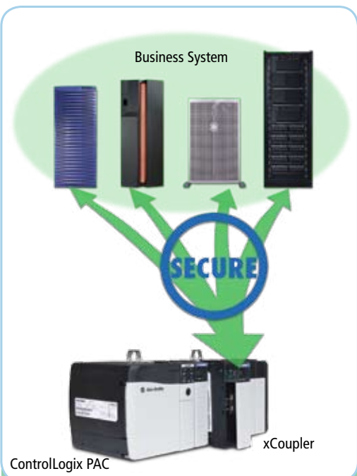
xCoupler module two-tier system in a PAC rack
